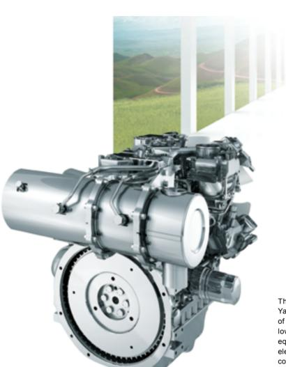
The P3504 is equipped with the Japanese Yanmar 4TNV88 engine with a displacement of 2.19L. It adopts natural aspiration and has low fuel consumption and strong power; It is equipped with a three-stage fuel filter with an electronic fuel pump; It has electronic flameout control system.
