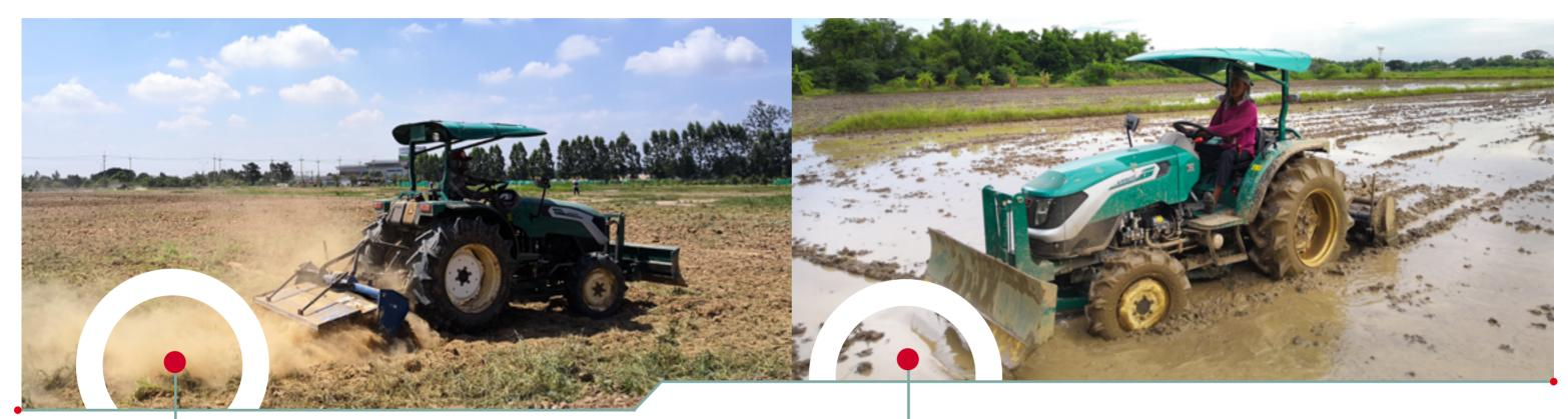
Overall working condition in dry fields: matching disk harrow, rotary tiller, front bulldozer and other machines and tools to easily complete stubble ploughing, harrowing, rotary tillage and other field operations.
