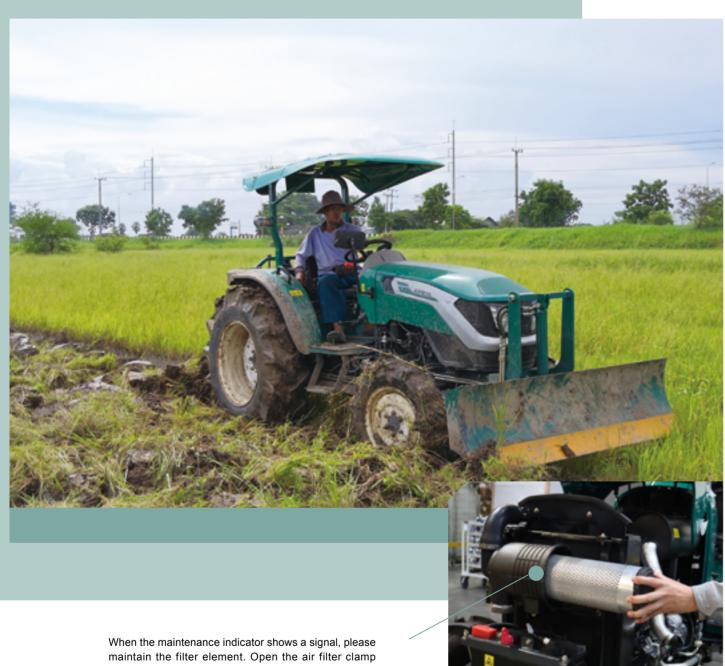
to remove the air filter cover, remove the coarse filter element and the fine filter element in turn, and blow it from the inside out with compressed air (pressure not greater than 588KPa). After the filter element has been serviced six times, replace it with a new one.
