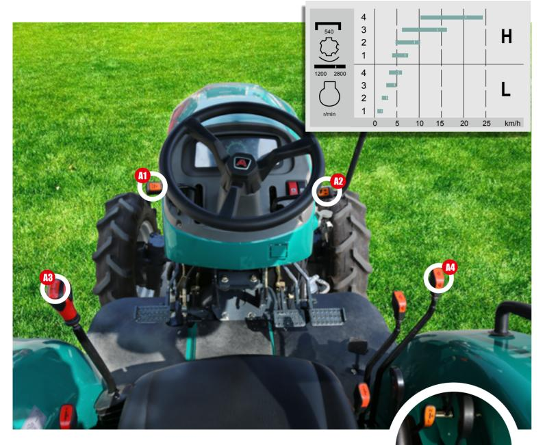
The distributor operating mark facilitates the user to judge the position of the machine and tools, that is, different lifting height correspond to different scales heights, and the use of limit knob can ensure the consistency of the working depth of the machine and tools.
